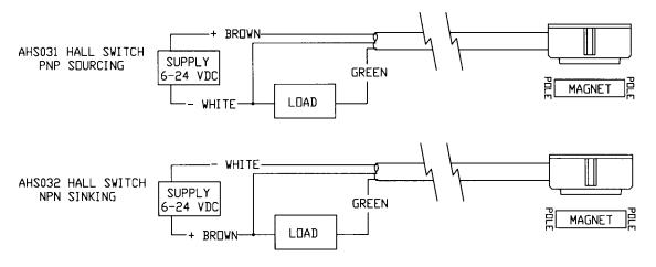
SHOWN WITH OPTIONAL ARC 130 8mm THREADED QUICK CONNECT CABLE
